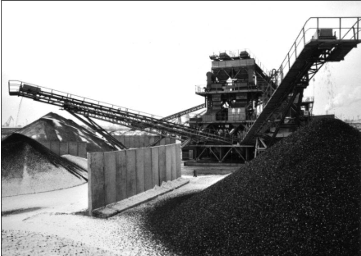
Fig. 11: Gravel scrubbing and separating machine
